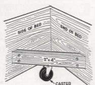
To install ball-bearing casters on your bunk bed, set a 2 by 4 across inside corner of bed frame. Place 2 by 4 far enough from corner so that, when easter is inserted, wheel can turn freely in any direction-and bunk is 34 in. above floor
