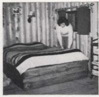
We simply installed ballbearing casters. Now even a child can push the large, double bunk away from its wall. Casters facilitate cleaning under bed, too
