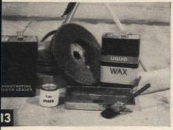
(13, 14) Floor sealer, oil stain, polisher, pan, small brush, wax, lamb's wool applicator applies the finish selected for this particular floor. (14) Carefully sweep up dust, then with brush apply sealer, mixed with stain as desired, along edges
