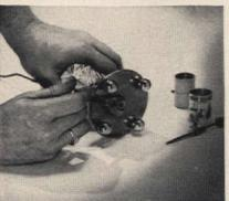
Reassemble lamp sections over central pipe and tighten snugly. If harp is plated or painted steel, re-gild, using gold bronzepowder mixed with lacquer. Use as thin a mixture as possible without running
