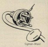
ends. Scrape wire clean and twist the strands together. Tie an underwriter's knot at the base of the split in the cord and pull it against the plug shoulder. Run each wire clockwise around a prong and a binding screw. Be sure there is no contact between bare wires, and slide the fiber shield over the prongs.
