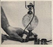
Rewire with old cord or new one if necessary. Loop bared ends of wire around terminal screws in the socket, and in direction they are to be turned. Tighten securely, install insulated sleeves and shell
