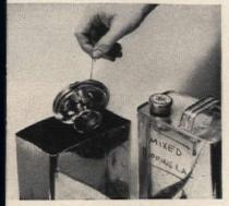
While still wet with thinner, place parts on hooks and dip into 50-50 mixture of lacquer and thinner. Remove and drain excess back into tank. Hang up to dry. Repeat
