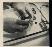
Buff parts with a "cotton wheel" on electric polisher loaded with tripoli. Finish with another buffing wheel and jeweler's rouge. Don't handle polished surface
