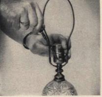
To start dismantling. slip end of a screwdriver between socket shell and cap. Separate. Work gently, avoid bending thin metal parts
