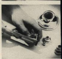
All traces of polishing compound must be washed off in thinner. Use soft cloth and brush to get down into crevices. Do not handle polished surfaces more than necessary
