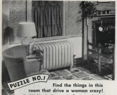
An old-fashioned radiator, wasting floor space-slow-heating, inefficient. A dust-collector that throws too much heat to the ceiling, not enough near the floor. It's too hot for you or your furniture to touch. Heat wasted. Fuel wasted. Trane "Active Air" Convectors would whip these problems.
