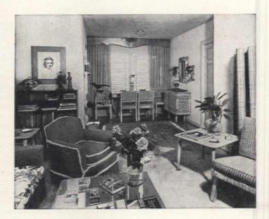
O Decorator West salvaged aluminum from scrap heap to make long valances across end of room. Cut with tin shears, border design is punched from reverse side with nail. Shaped board is backing
