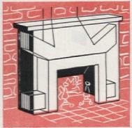
Heat circulator in fireplace will supplement the radiant with convection heat for more comfort
