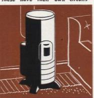
Some oil heaters have burners equipped with a blower. Others operate by gravity air flow
