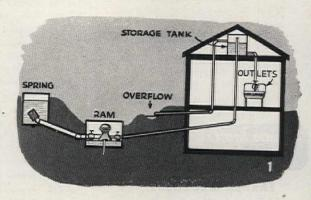
Four different types of water systems for the country. 1) A Spring and ram system. Hydraulic ram requires no electric power to operate.
