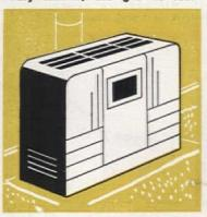
Oil heaters may use No. 1, 2, or 3 grades of fuel oil, depending upon the design of the burner
