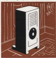
Oil space heaters, like this one and the next two, require a flue. Many different types are available
