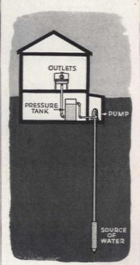
Most reliable type of water supply is the artesian well, described in text. Deep well pump and pressure tank are required with this system
