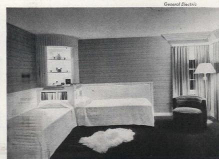
Fluorescence built into table gives reading light for beds in modern room. General lighting from ceiling fixture
