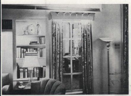
Direct lighting, indirect lighting, separately or together, are possible at valance in General Electric's Horizon House
