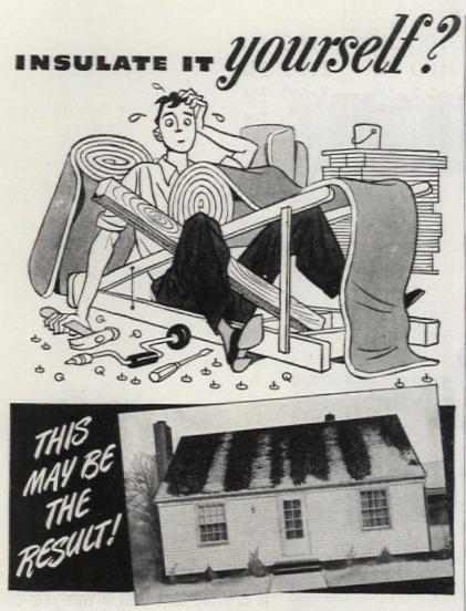
Here's dramatic proof that "Insulation is no better than the man who installs it"! Those streaks of snow on the roof tell the story. Inefficiently installed insulation permits heat to pass through part of the roof—melting the snow—sacrificing both fuel and comfort.
