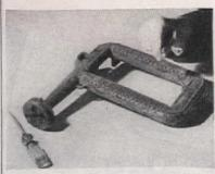
Use a piece of wire to clean clogged holes in oven burner and in the four top burners
