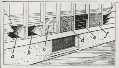
Insist on ratproof construction; (a) a common type, is not. Effective devices are firestops (b), sheet of metal (c), a fill of cement and cinders (d), bricks (e), or, best of all, rich concrete (f)
