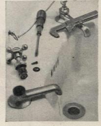
Removal of small screw at base of stem frees old washer which is reversed or, better, replaced
