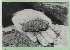
Proper soil, squeezed, will hold its shape, but crumble if dropped
