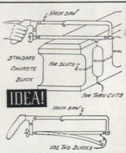
SAW CEMENT! A standard size concrete block (8"x8"x16") can be cut with an ordinary hacksaw fitted with two or more blades. This can be done without danger of cracking the entire block, which often occurs when a chisel and hammer are employed for this purpose, as is so frequently done.-H. D. YOUNG
