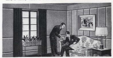
The secret of Mr. Hamby's wall design lies in using panels of Tempered Presdwood with a combination of interesting joint treatments in which the panels are separated by fluted wood sticking. Notice particularly the deep, soft shadows between panels. The edges of the Tempered Presdwood may safely be nailed or glued to the sticking because this grainless board does not warp, chip, split or crack when applied according to instructions.
