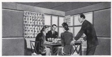
· Here in the "dining" end of this smart living room-dining room unit, Mr. Hamby has made horizontal Tempered Presdwood paneling the predominant note in wall treatment. Tempered Presdwood can be cut or sawed with ordinary tools. It can be painted, enameled, waxed or left natural. Its marble-smooth surface is unusually easy to keep clean, and the board is as permanent as the building itself. Mail coupon below for free sample.
