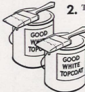
2. Then apply usual two topcoats all over and the paint will normally wear uniformly and keep looking the same, on vulnerable places as well as on the rest of the house. Repainting will not be needed so soon.
