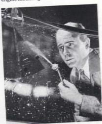
Wiper Tests—Not only the mechanism but the rubber is tested as in the many other parts of the car where this material means long life.
