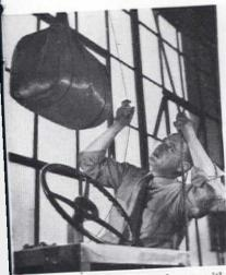
Rubber He Can't Break even with this 200-pound weight. Plymouth's sturdy steering wheel is made of hard rubber, with a solid steel core.
