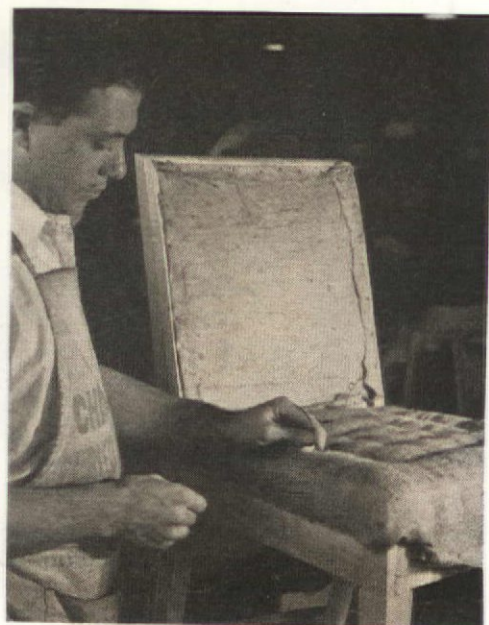
Hair filling is firmly stitched to 5. burlap. Careful handwork plays a large part in this and other steps
