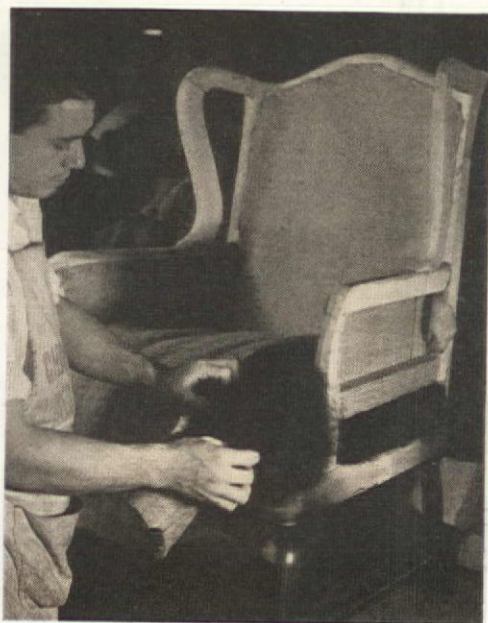
A thick, even layer of horsehair is 4. spread over the burlap. Beware of the cheap substitutes for horsehair
