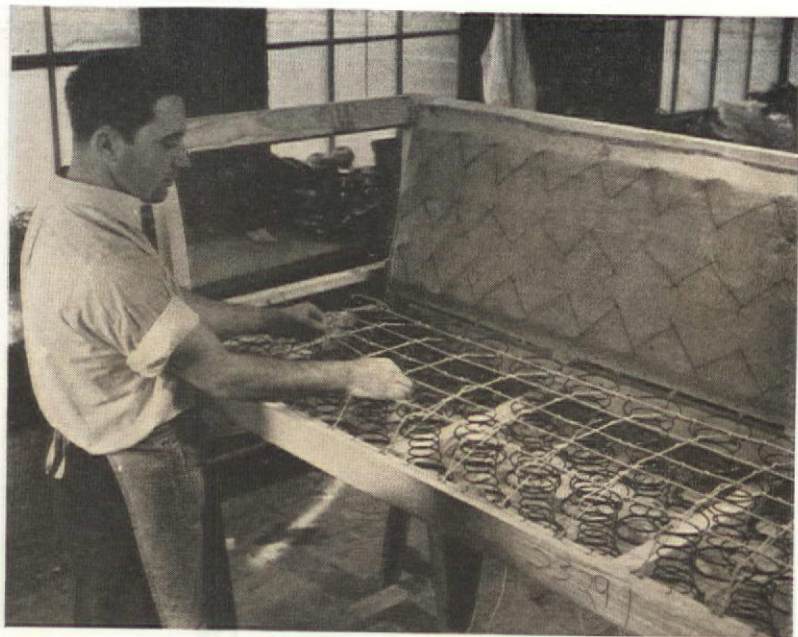
Oil-tempered steel springs are knotted on both ends, so they can- 2. not break through and tear the upholstery fabric. The springs are fastened together with strong twine, tied eight ways by hand
