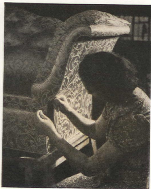
Finally, the exterior upholstery fa- 8. bric is sewed on by hand. Care and skill make a finished-looking piece
