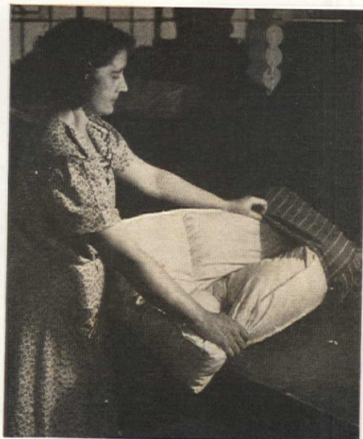
Down-proof muslin casings, divid- 7. ed into compartments, prevent bunching and slipping of filling
