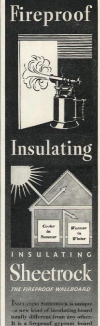
It is a fireproof gypsum board equal in insulating value to a full half inch of fiber insulating board. The inside surface is the standard ivory color of Sheetrock that takes any type of decoration. But the opposite side, that is placed next to the building framework, is actually a thin sheet of aluminum foil which acts as an efficient insulator.
