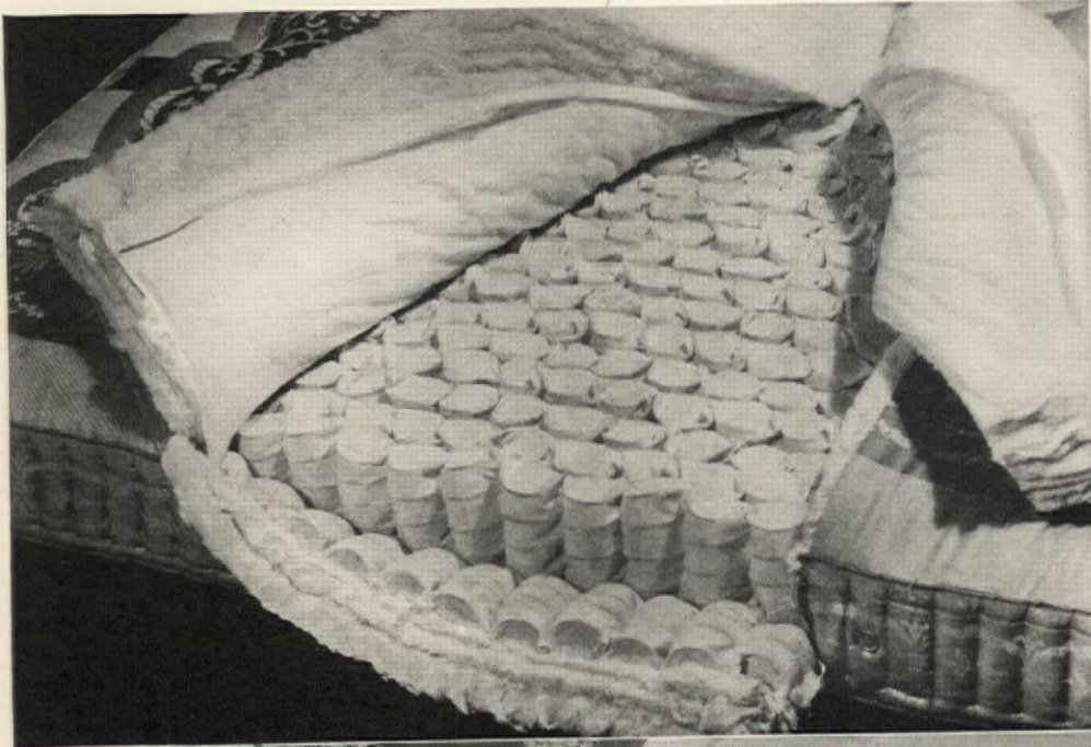
In this type of mattress of the multiple unit innerspring construction the coils, individually pocketed and arranged in nests, are tied in occasional places to allow for freer action and resiliency. Below, section of a box spring showing the intricate system of tying the coils in position (The Simmons Company)
