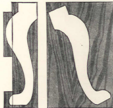
Cabriole or curved legs, regardless of size, where used should be in one piece. To economize on wood they are cheaply cut from a straight plank with blocks glued on to take care of the projection of knee and toe in the cabriole and to allow for the wide swing of a curved leg of any type. Look here for solid construction
