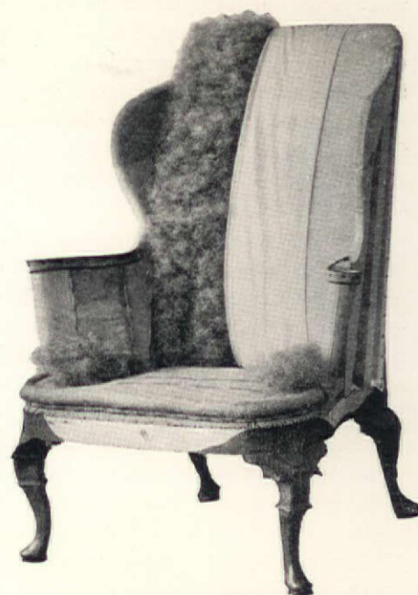
Cabriole or curved legs, regardless of size, where used should be in one piece. To economize on wood they are cheaply cut from a straight plank with blocks glued on to take care of the projection of knee and toe in the cabriole and to allow for the wide swing of a curved leg of any type. Look here for solid construction
