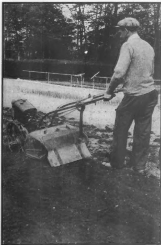
Direct application of power to pulverize and mix the soil for crop preparation is made in rototilling. The worked area is "offset" so the operator does not tread on it
