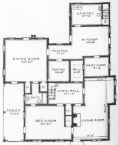
The first floor plan of the remodeled old house is shown at the right and above it is the layout as originally found. Note that the partition was taken out to increase the size of the living room, and a fireplace installed
