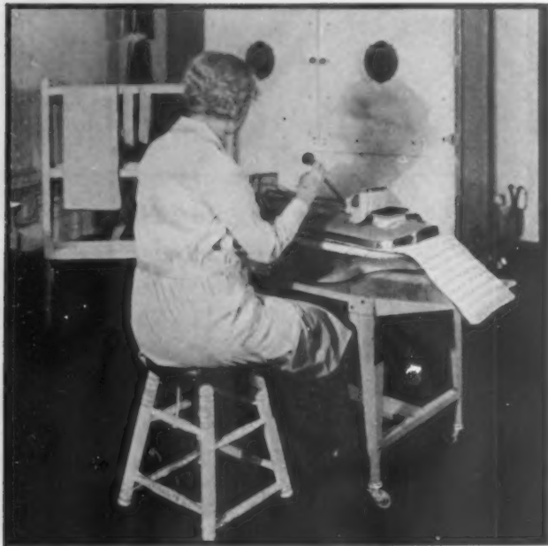
Pleated dresses, ruffled curtains, shirts, even men's suits may be turned out with a professional finish on this machine which is controlled by a hand lever. (All Meadows Press Ironer)
