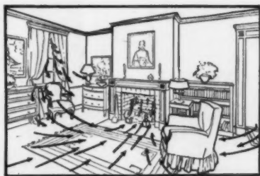
Old-style fireplace. Chimney draft draws cold air into house. COLD, it drops to floor, chills it and passes up chimney. No ventilation. Cold house.
