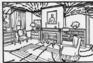
Bennett Bonded Fireplace. Fresh outdoor air drawn through fireplace and warmed. Circulates to other rooms. Full ventilation and effective heat.
