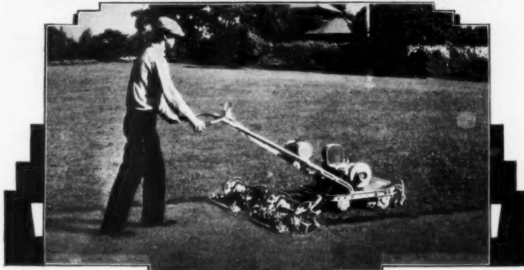
Above: Coldwell "L-Twin" motor lawn mower and roller. Mows and rolls 4 to 6 acres a day on one gallon of gasoline. Gang units more than double its capacity.
