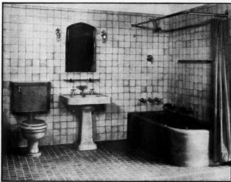
This modern bath has a floor of rose tile, tub and other fittings of pale sea foam green, walls a dull ivory tile, with a rose shower curtain. The plumbing is of chromium, and therefore non-tarnishable. (Courtesy C. F. Church Mfg. Co.)
