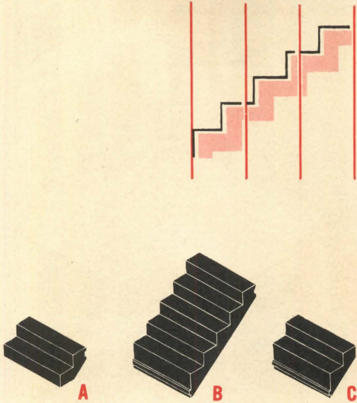
BASIC STAIR UNITS. FROM THESE UNITS, ANY OF THE COMBINATIONS SHOWN ON THIS AND THE OPPOSITE PAGE, AND MANY MORE BESIDES, CAN BE MADE UP.
