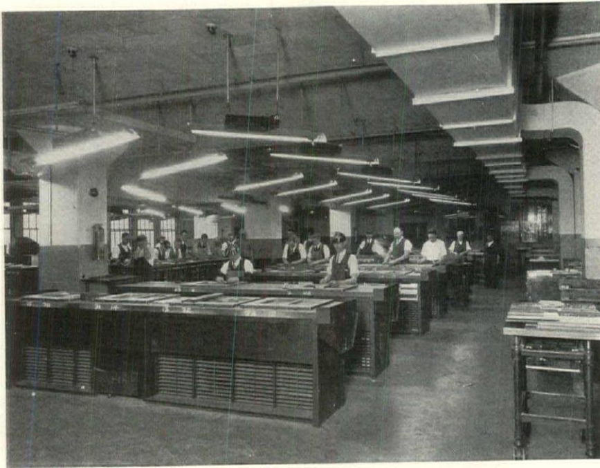
Composing room showing make-up tables for page forms. Sound-absorbing covering on the ceiling
