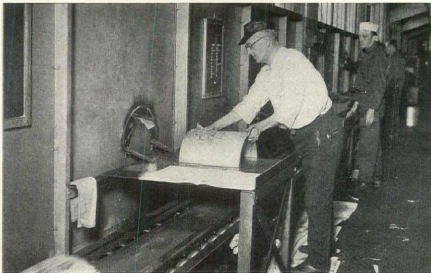
Receiving the plate in the press room where it is placed on the conveyor, under the table, to be transported to the presses
