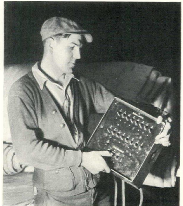
Portable Control Board for Bank Lights
