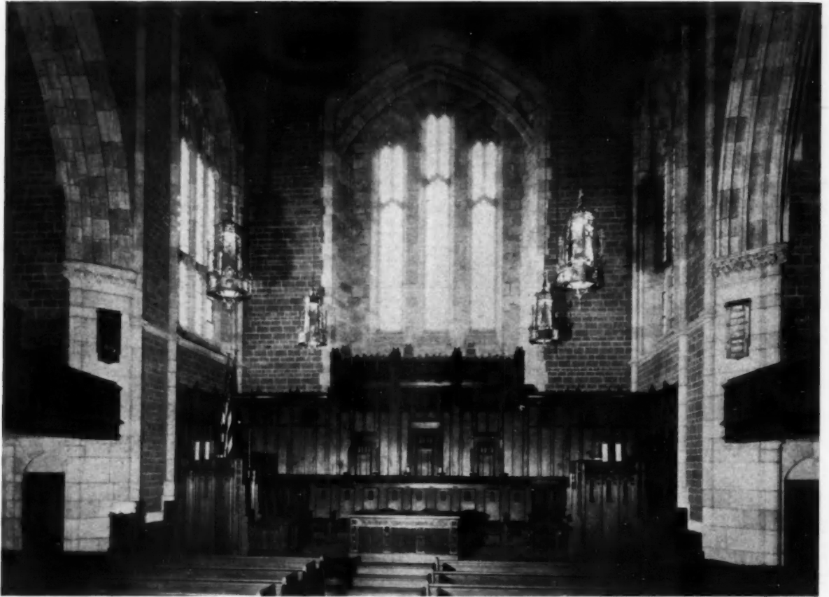
Fig. 14. Cushions and Sound-absorbing Tile Control Reverberation Bryn Mawr Presbyterian Church, Bryn Mawr, Pa.
