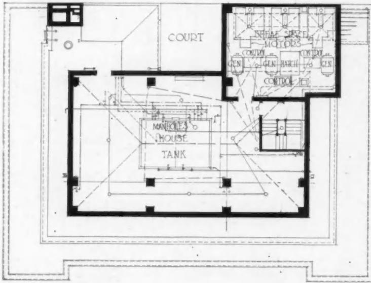
Plan Showing Elevator Machinery and Tank in Penthouse on Roof,
