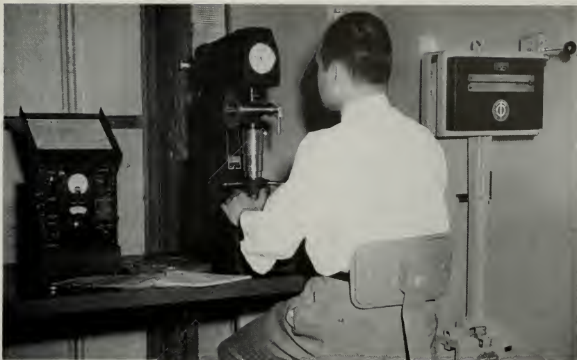
New Mechanical Laboratory showing Research Engineer A. V. Engle using a testing device to determine the hardness of a machine part produced in the Southwest Research Institute's shops. At left is shown instrument used in conjunction with strain gages for measuring changes as small as .00002-inch and (right) is a machine which determines the resistance of various metals to compact loading.
