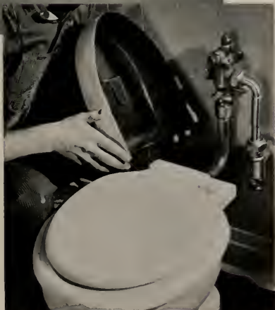
The streamlined housing which covers the flush valve is easily removed for inspection. The entire combination is compact and space-saving, roughing-in normally at 10" with ample tolerances for both water and waste connections.
