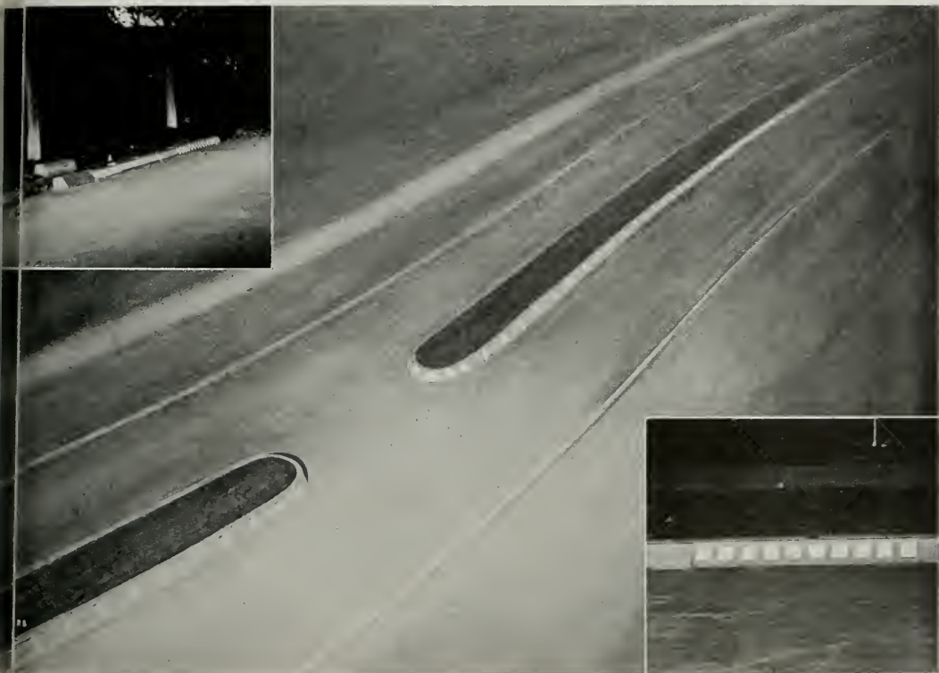
Artist's conception of new type of reflecting curb for intersectional islands and division strips. Upper inset shows wedge shaped recess for separation strip curbs. Lower inset shows block type recess under direct headlight rays.
