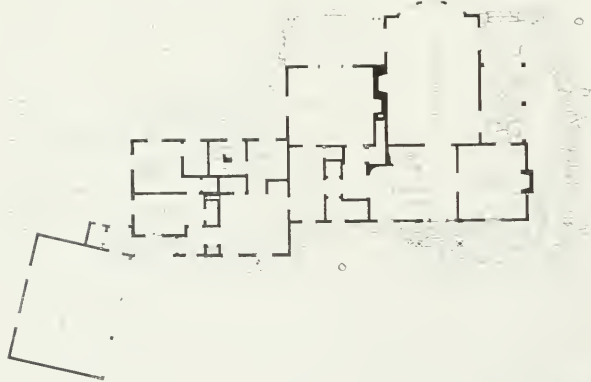
First floor plan. Note living quarters well separated from kitchen, laundry, servant's room and garage, assuring owner the privacy of his family.
