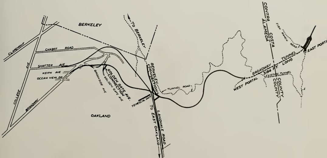
Sketch map shows location of Broadway Tunnel and Berkeley connections. Old Tunnel Road shown by wavy dotted line.
