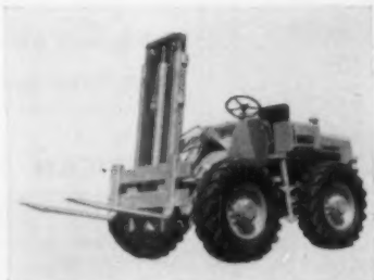
FORK-LIFT TRACTOR is the same basic 4-wheel drive machine as the tractor-shovel. Capacities up to 6,000 lbs; lifting heights up to 21½ feet.
