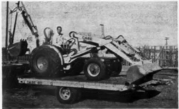
RIG MOVING —Tractor fitted with front-end loader and backhoe is loaded on Case trailer ready for haul to new job. Complete rig, fully mobile, enables builder to do his own work yet take on many subcontractor jobs which add to profits.
