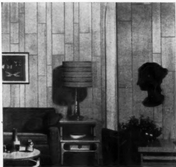
LOC-WALL: Idaho White Pine and Inland Red Cedar in Formal and Traditional styling; Larch in Formal styling. Plywood Panels look like individual boards of random lengths and widths, edge and end-Vee'd. Also produced with Gruve-Ply pattern. Interlocking furring strips are already attached.
