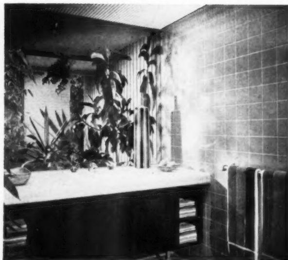
12 THE GLARE IS GONE. Plastics have come into their own for bath use, and they're ideal for diffusing light. In the L. A. Times house, Infilite is used for the ceiling. Available in 24x25" panels, it's interlocked so no joints show.
