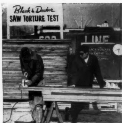
8:30 A.M. Over twenty-two hours of work and a third shift of technicians. The B&D Saw is as fresh as a daisy although it has used 13 blades to this point.
