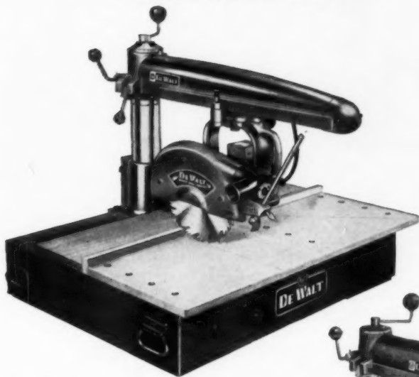
MODEL GW-1 WITH 10" SAW. With 1½ hp direct-drive motor, 120/240 voltage change switch. 10" saw blade cuts 3" deep, rips 26" wide, cross-cuts 16" wide on 1" stock. Steel base with welded carrying handles, carries through 30" door. Safety key switch, guard, anti-kickback device. Weighs only 183 lbs.
