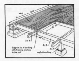
2.4.1 is both subfloor and underlay. Inset 2 x 4 blocking supports panel edges. Drawings below show how girders set flush with footings improves appearance by lowering house about 12 inches.
