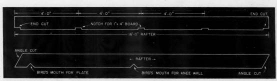
TYPICAL GANG JOBS are ceiling joist, top, and rafter, below. Joist requires five dado heads, the end ones
