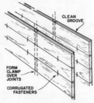
Instead of the conventional battens and common nails, I use corrugated fasteners only.
