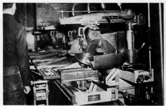
THIS GANG of five radial saws is making short work of a rafter. Air cylinders operate both the saws and
