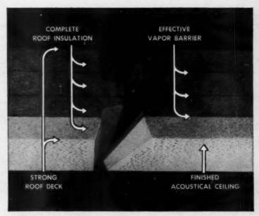
New Armstrong Cushiontone Roof Deck is a 4-in-1 material that provides roof deck, complete insulation, multiple vapor barriers, and finished acoustical ceiling in one fast, simple application. It needs only beams to support it and built-up roofing to weatherproof it.
