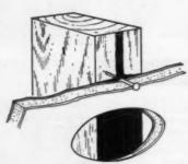
CUT-A-WAY shows how bead is spread to 1/16" bed. Cushioning effect of bed reduces nailhead fracturing of face of paper. Continuous bond bridges framing irregularities.
