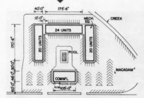
TESTED plot plan shows excellent arrangement of parking around motel units as well as the commercial building. This additional parking allows travelers who don't intend staying overnight to get in and out easily.
