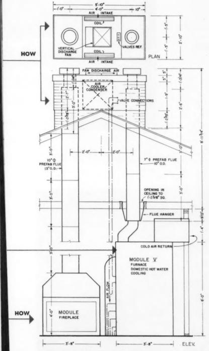
NEATNESS and compactness of the entire heating system is shown in this drawing. While the greatest economy of space is attained with the spacing here, the flues are sufficiently flexible to allow the fireplace and heater to be shifted around to a limited extent.
