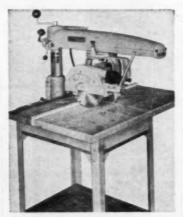
TABLE OR BENCH SAWS are rated high for shop work, heavier cutting jobs. Above, a radial-arm woodworking and metal-cutting saw. From De Walt (No. F55, p. 124).
