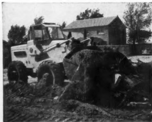
SPECIALIST in loading is this Hough "Payloader". Big rubber tires give it speed and mobility, let it run on highways. (No. D45, p 108).
