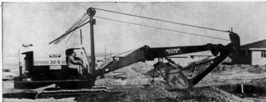
CRANE —excavator combination is this new unit by Bucyrus-Erie. The type 30-B crawler unit can be fitted
