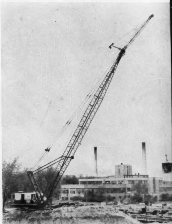
CRANE BOOM handles concrete bucket, can also swing drag-line bucket. Similar, but smaller boom can be used on the smaller machine below. Both would pay off best in big scale land development.
