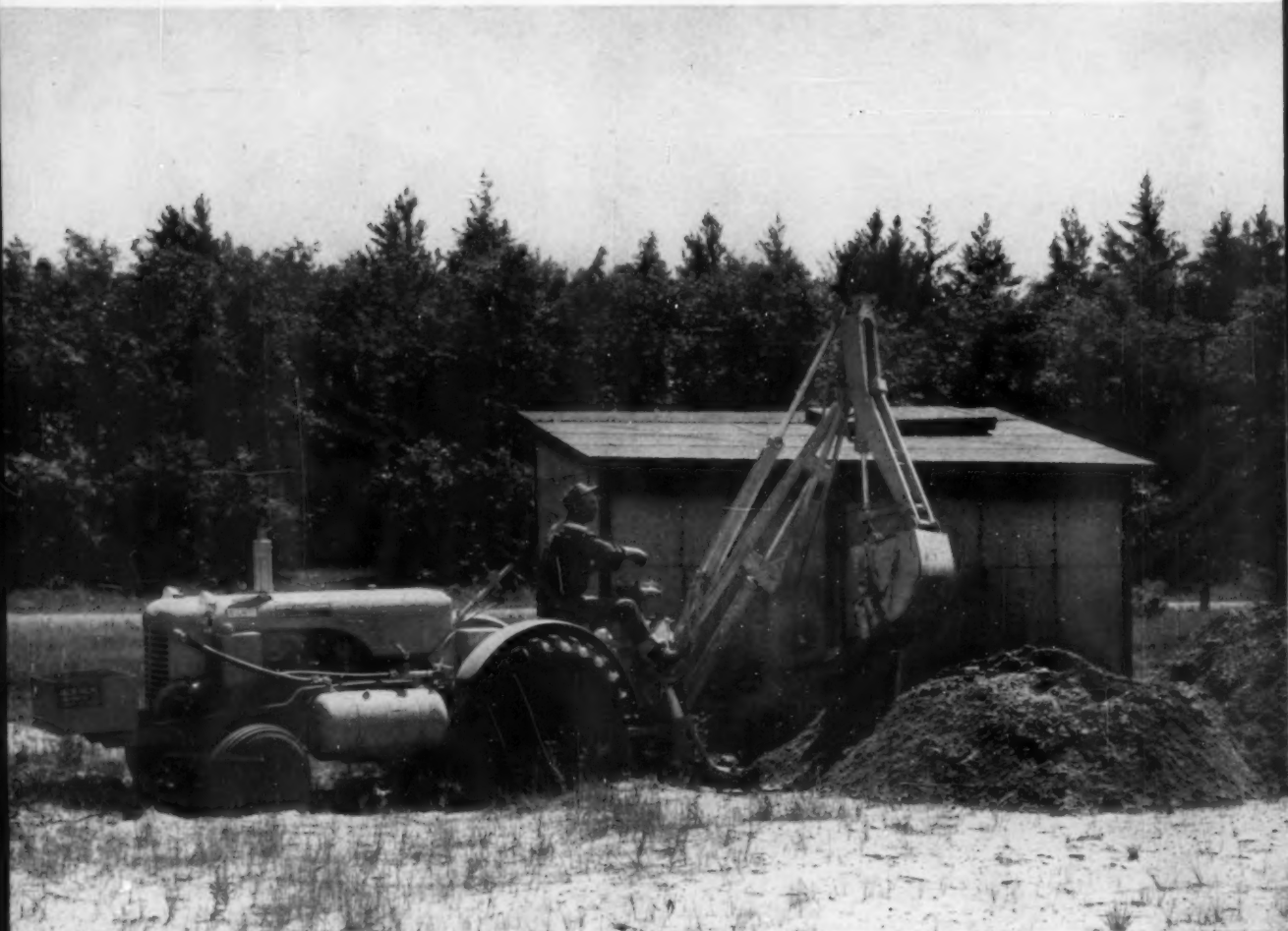
BESIDES standard attachments such as backhoe, this Le Roi "Tractair" carries its own compressed air for pneumatic tools and attachments. (No. D44, p 108).
