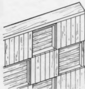
CHECKER PATTERN. Frame with short 2x4" girls toe-nailed to 2x4" posts. Cover squares alternately with short 1x4" V-edge siding (shiplap or T&G). Bruce Heiser, Architect.
