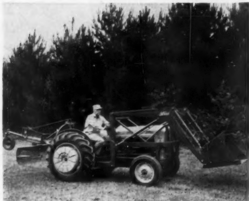
IDEAL COMBINATION for light grading and landscaping is this Ford tractor with front-end loader and adjustable rear blade. (No. D47, p 108).
