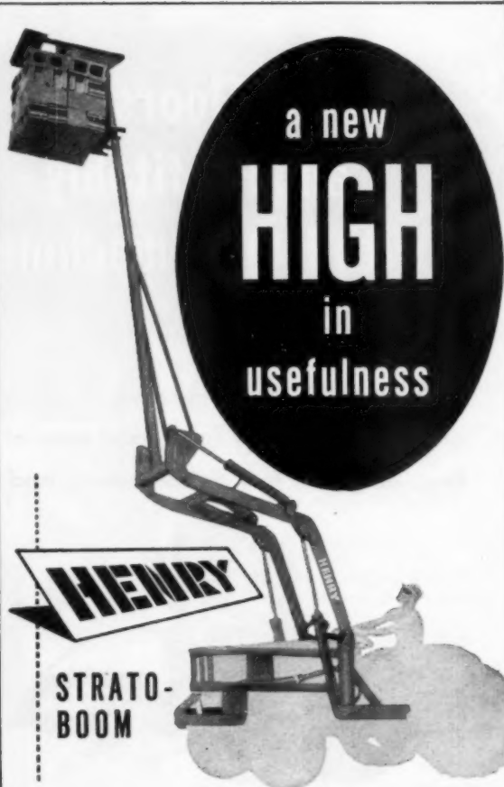
MODEL 360-57-90 — Half-yard; 360° continuous swing. New 90 GPM hydraulic system with triple tandem pump and split valve bank. For truck or carrier mounting.
