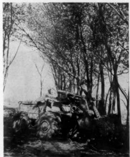
MEDIUM-SIZED DIGGER is set up on a rubber-tired tractor, better for road travel, and finished landscaping.
