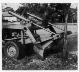
STARTING TO DIG UP the tree. See how the bucket shape allows working without damaging the tree trunk.
