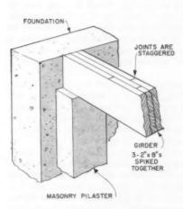
A s a general rule, a girder, or girt, will run down the approximate center of the house on the long dimension. On narrow houses it is sometimes possible, with the use of extra heavy joists, to avoid the use of a girder, but in the house shown here, it would be necessary. And even on the narrow house, there might be too much deflection if the girder were not used.
