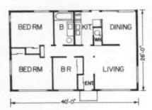
The house to be used as the example in estimating framing costs is shown at the left. It is a gable roofed, one floor home with three bedrooms and one bath. It is built on a crawl space or a basement—the framing cost will be the same in either case. If it were a slab model, the sill would be figured, and then the flooring would be skipped altogether and the estimate picked up again at the sole plate.
