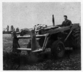
HOLE IS DUG in the new location, will be just the right size to accommodate the earth ball on the tree.
