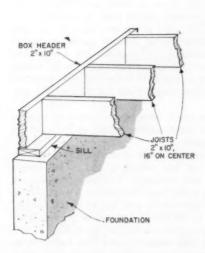
Joists sizes will be determined by their span and their spacing. For the house in question, 2x10's will be used, spaced on 16-inch centers. The box header is nailed across the ends of the joists on the long dimension, and provides stiffness and a nailing surface for sheathing and siding.
