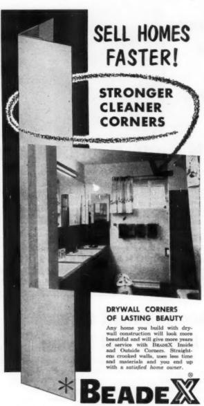
BeadeX corner beads offer you exclusive advantages over other types of bead...BeadeX is applied directly to the wall surface, expanding and contracting in direct ratio to the wall material. No unprotected metal to rust.
