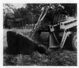
SMALL BUCKET is shown here mounted on the front end of a small tractor. It is used to handle smaller trees.
