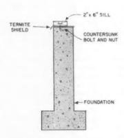
The sill is generally made of 2x6's bolted to the top of the foundation wall. It should be set flush with the outside edge of the foundation, so that the sheathing and siding can lap down over it and insure against water being driven in between the sill and the foundation.
