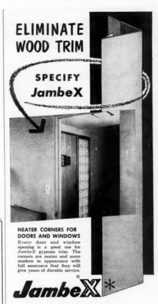
A combination metal and paper trim that adheres to the drywalls itself to overcome cracking from stud or frame movement. JambeX is applied directly to the walls around doors and windows and inserted in a sawed kerf in the jamb stock. JambeX corners are quality corners that remain straight.
