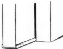
ALUMINUM GUIDE STRIP ATTACHES TO BOTTOM OF DOOR . . . GUIDES DOOR INTO POCKET
