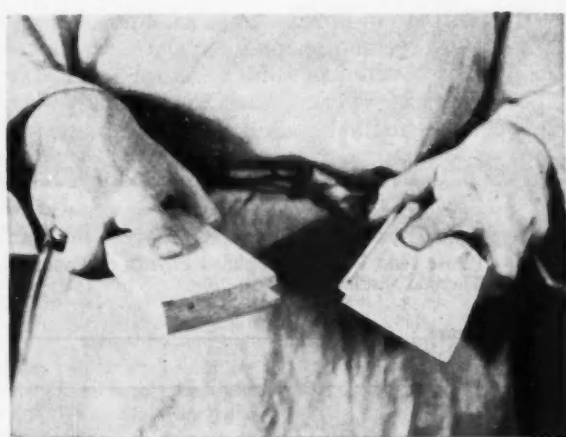
EXAMPLE of the tongue and groove that can be run on a radial arm saw equipped with a safety power feed
