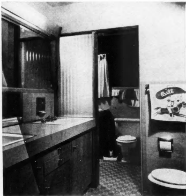
OBSCURE GLASS in panel reflects light to second unit of compartmented bath
