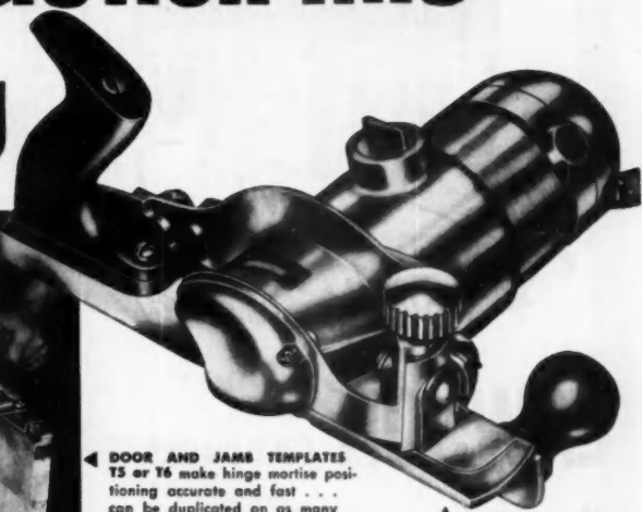
▲ ELECTRIC PLANE, J38 Completely new! Does fast, flawless trimming and fitting of doors. Ingenious design of housing blows chips entirely free of cutter. Planes widths to 1 3/4". Bevels 45° outboard, 15° inboard.
