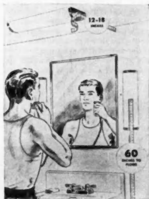
TESTED lighting results are assured when builders follow simple and easy instructions for bathroom lighting as developed in lighting laboratories of manufacturer
