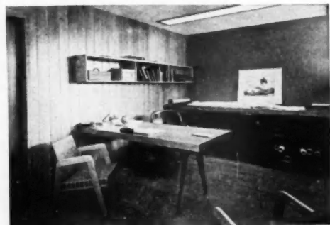
CHIEF architect's office has asphalt tile floor, acoustical ceiling and one of the walls is paneled in golden oak
