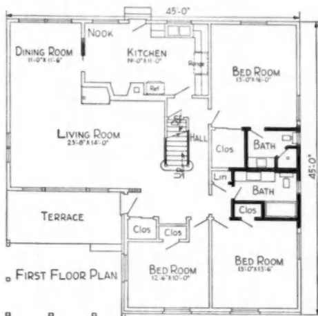
"BACK-TO-BACK" arrangement of plumbing for the two bathrooms shown in plan above is economical
