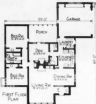
"MIDWEST HOUSE" floor plan. Alternate plan provides basement, converts utility space into basement stairway and closet for den
