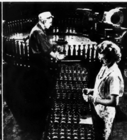
HERE KNOBS are leaving the 12-foot polishing dial. Note how they sparkle. Inspector is near operator checking units
