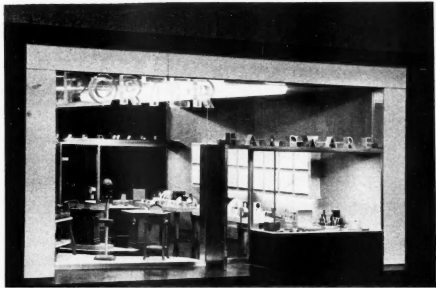
GRAY AND BLUE structural glass have been combined in this front. In an effort to create the illusion that there is no glass separating the exterior from the interior, the gray of the left base was carried into the store interior as a wall covering
