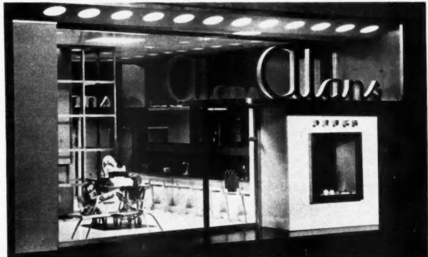
THIS DRUG STORE was planned with a feature display element at the street end of the counter to block off the unattractive view inherent in behind-the-counter soda fountain operation. Main plate glass display window here is set at an angle in plan
