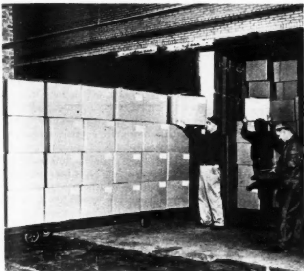
5. COTTON insulation, compressed tightly for shipping or storage, quickly regains thickness when unrolled
