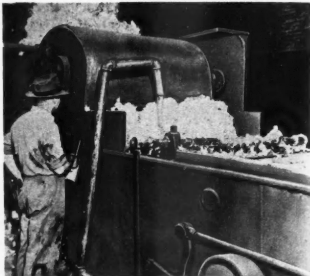
1. VIRGIN, fleecy cotton goes through flameproofing bath as one of first steps in manufacturing cotton insulation
