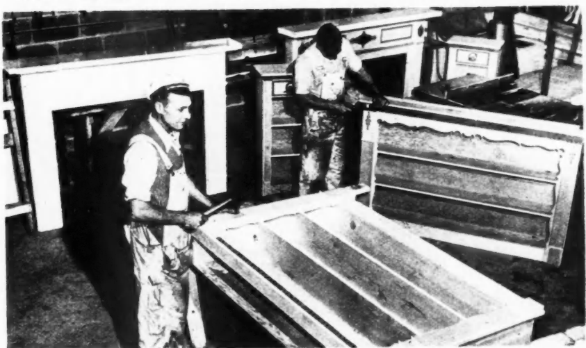
PORTION of shop, showing mantels and built-in bookshelves in process of manufacture
