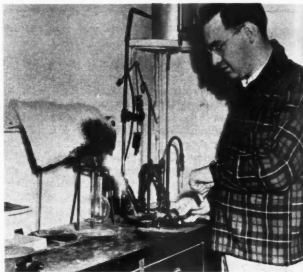
4. SAMPLES of insulation are submitted to 1800-degree test. Surface blackens; does not burn
