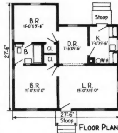
PLAN B is a variation of plan A. Compact and efficient arrangements were used in project's kitchens and bathrooms
