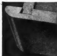
DOVETAILED DRAWER FRONTS The dovetail can only be seen from the bottom—doesn't come up through the top—where it would detract from appearance.
