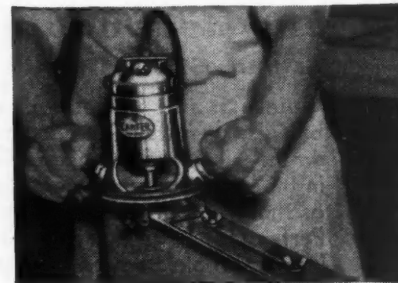
Hinge Butt Router HB4A. With door and jamb templet this 3/8 H.P., 18,000 R.P.M. router can mortise 75 doors and jambs a day, accurately. No shimming or recutting. Also used with lock face templet.
