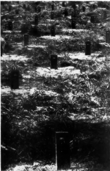
Accelerated tests with specimens of wood, buried in heavily infested ground, are continually checked to show effectiveness of Monsanto formulations.
