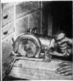
Cutting Dadoes or Grooves of any width is quick work with Grooving Blade.
