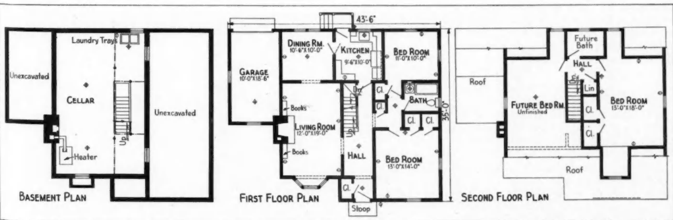
THESE basic floor plans of Bulder Gustave Feuerstein's three trim Colonial homes on these pages present a good six- or seven-room arrangement with center hall and unfinished second floor bedroom and bath. Basement is unexcavated under the garage and bedrooms.
