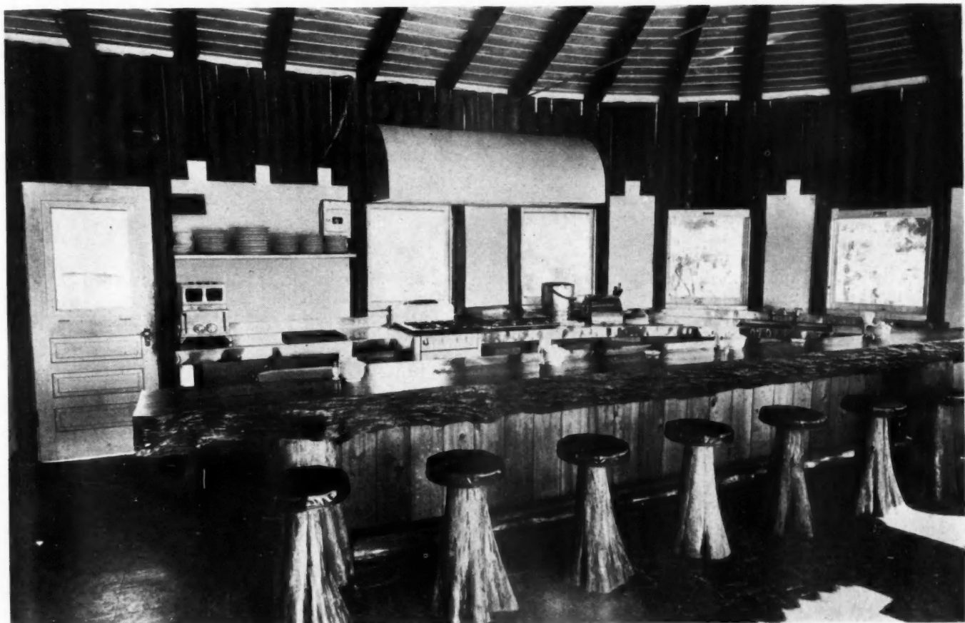
A 2,000 POUND EVERGLADES LOG sawed into a slab 22 inches wide is used for the counter top in Scottie's Coffee Shop. Cypress stumps are used as stools. Kitchen equipment is of stainless steel.
